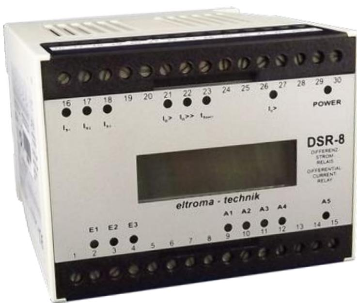
The DSR-8 is a device for measurement and monitoring of differential current at generators, motors and transformers. As well possible is the monitoring of mixed constructions, such as a generator with an upstream transformer. In addition to the differential current, it is also possible to measure the individual conductor currents as well as the earth current in three-wire networks. The connection to the system must be done using external current transformers.
